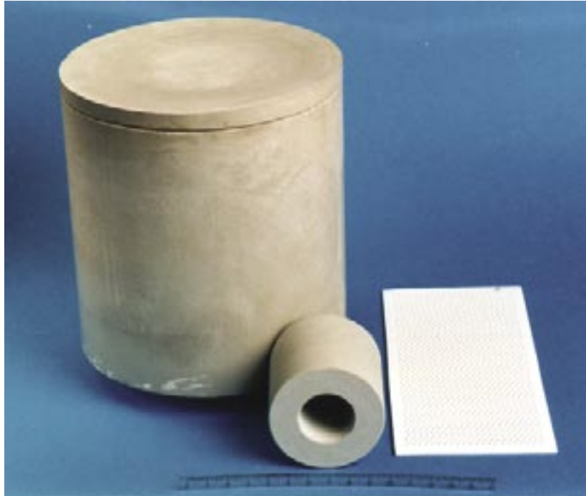
Both starch consolidation and protein forming offer good opportunities to shape components with various sizes and shapes.
