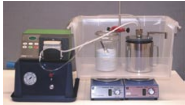
Lab-scale freeze granulator (LS-2, PowderPro AB).
